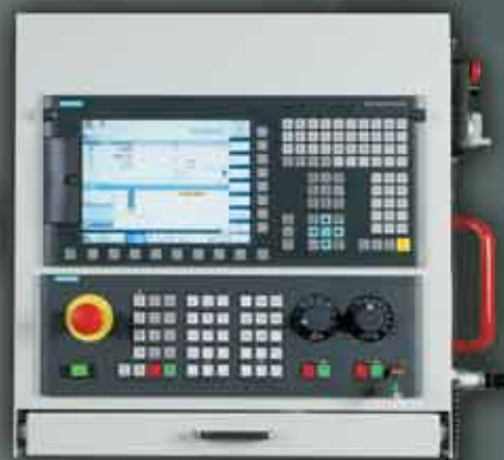
SIEMENS 828D Control with 10.4" Color Display and software: Shopturn
